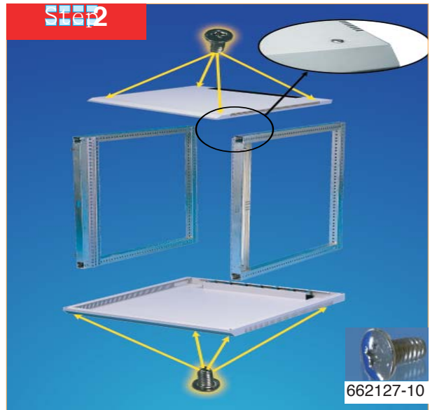
Step 2 Removing Mounting Angle Check Mounting Angle where you want .
