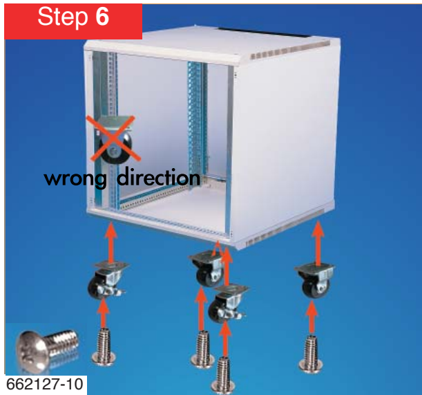
Step 6 Assembly Castor .
